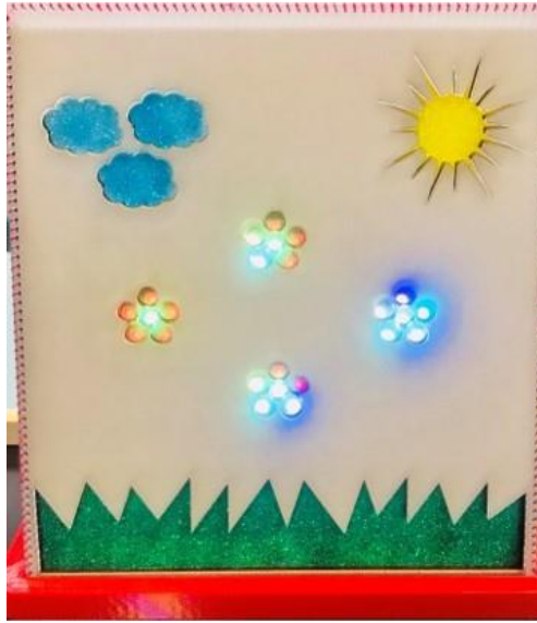
Figure 5: In this image you can see the final product of my FabAcademy project named MakerGarden. The lights are controlled by a mobile app. MakerGarden is created by using the most common forms of digital fabrication process: 2D design & laser cutting; 3D design & 3D printing; PCB design & production & programming; adding input & output device to the microcontroller board that I designed; and interface & application programming
