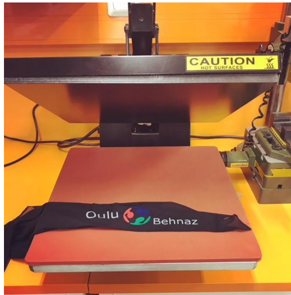
Figure 4: The Fab Lab logo and my name in this image are first designed in Inkscape (a vector graphic software), then cut on a vinyl material by using vinyl cutter, and finally printed on a piece of fabric using heat press machine (the machine shown in the picture).
